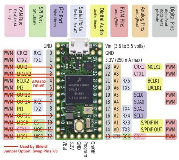
The additional pins on the right - 14 to VIN - are used to provide the additional functionality to the controller breakout.
